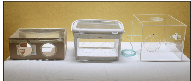
Fig. 1. Progression of the SAMPLAR box prototypes: prototype 1 (left): cardboard model for sizing and basic simulation; prototype 2 (centre): picnic basket and acrylic model for functional application and proof of concept; prototype 3 (right): fully operational final model with the inclusion of oxygen inflow port and access port covers (350 mm × 400 mm × 250 mm).
